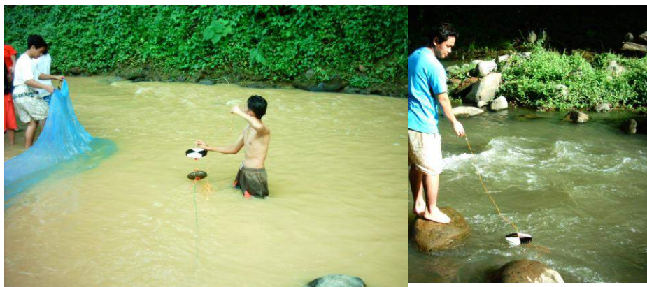
Student researchers measuring turbidity using the secchi disk
