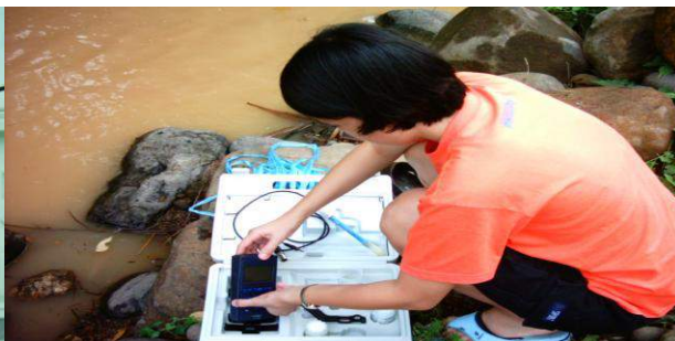
Researcher measuring the pH using the pH meter
